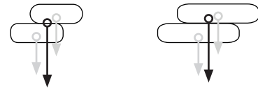
Fig.36 Wider layers provide stability and help printing steep over hangs
